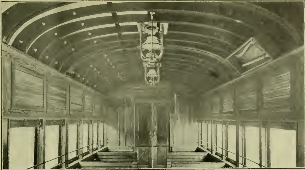
INTERIOR OF SECOND-CLASS PASSENGER CAR, WITH THE ROOF ONLY PARTIALLY FINISHED, SHOWING THE HOLES THROUGH THE CARLINES FOR CIRCULATION OF AIR IN THE ROOF.
